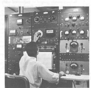
Instrument panel for a mass spectrometer
