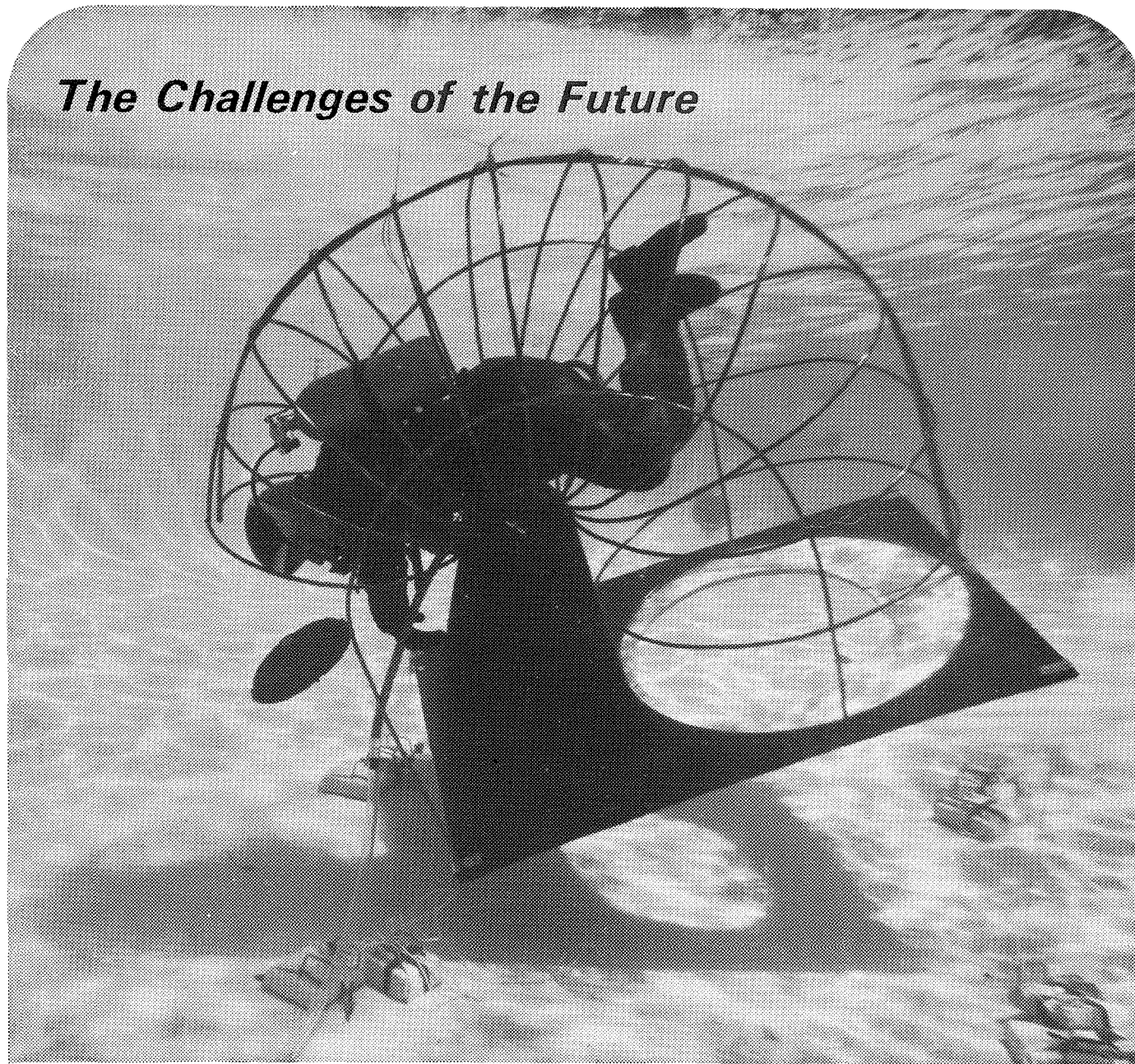
Challenge: simulation of activities under zero-gravity. Experiment: establish neutral buoyancy for astronauts in unique underwater testing sequence.
