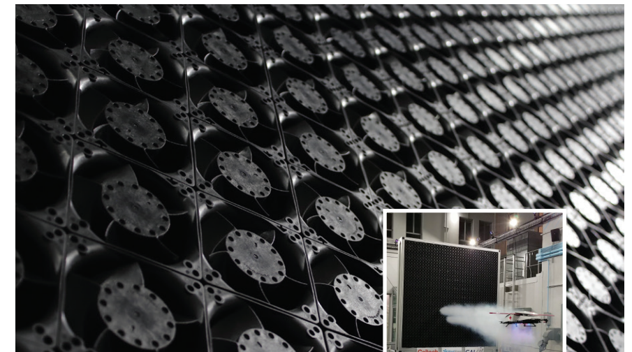
The fan array replicates a variety of real-world weather conditions for the model of the autonomous flying ambulance.
