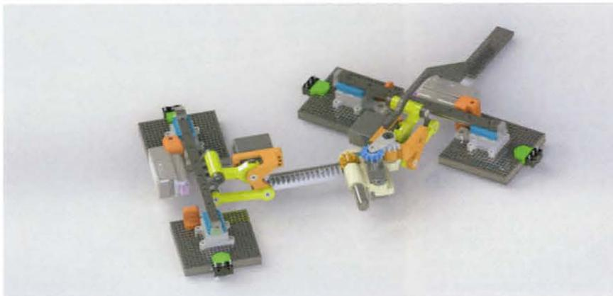
Figure 6: ACROBOT I used kinematically synthesized compliant 4-bar linkages to lift pads onto and off of the climbing surface.
