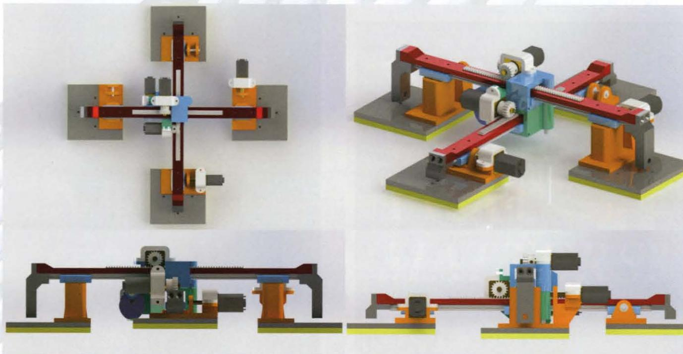
Figure 7: Top, front, right side, and isometric views of ACROBOT II. The top view shows all five of the actuators and their locations within the robot.
