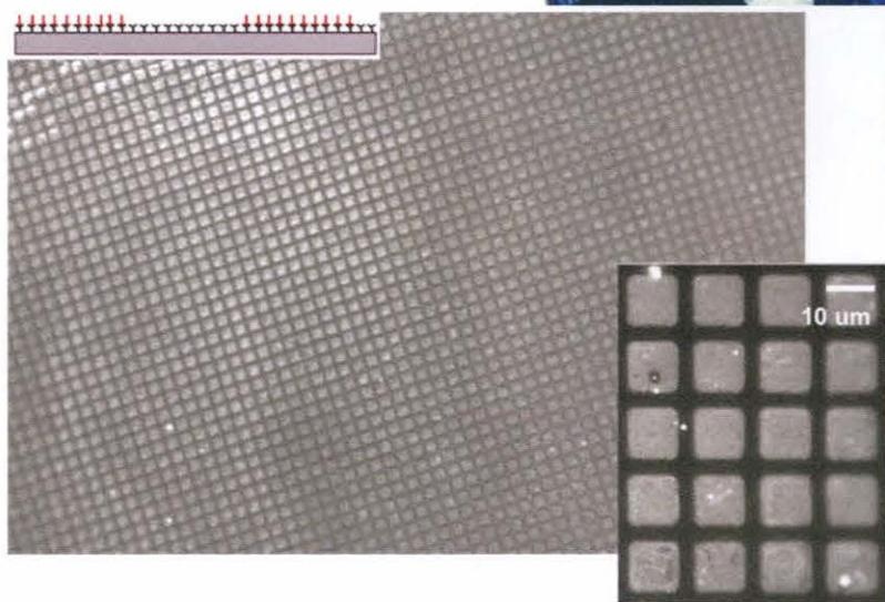
Figure 12. Fluorescent microscopy of biotinylated films stamped with strept-avidin AlexaFluor. While hierarchical patterns are not visible here, they are present due to the preexisting nanopatterns on the films. Pattern preservation of the stamp was preserved, indicating that this method could be used with any particle with strept-avidin.
