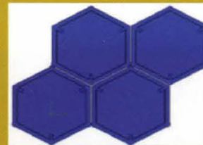
Figure 5: For FEM Analysis four unit cells represent the whole lattice due to symmetry
