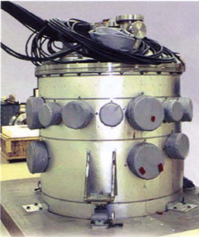
FIGURE 8 Picture of the Sustained Spheromak Physics Experiment (SSPX) apparatus. Plasma and magnetic fields are created in a toroidal arrangement within this structure. Source: David Hill, Lawrence Livermore National Laboratories.
