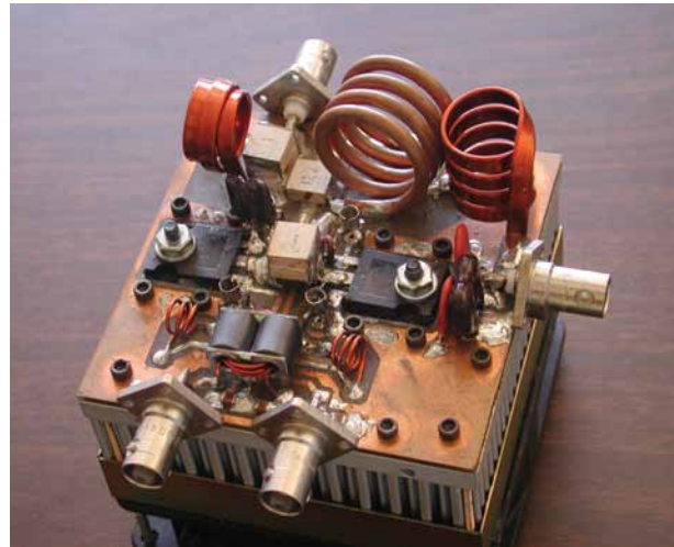
Figure 1: Prototype E/F switching amplifier developed by Scott Kee and Ichiro Aoki 1 . This amplifier produced 1.1 kW at 7 MHz with 85% efficiency.
