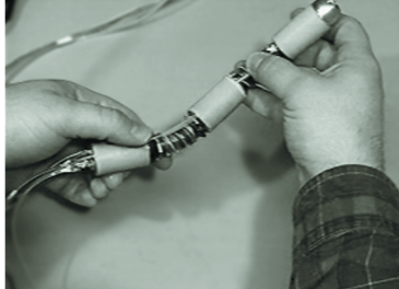
Medical robot prototype. The goal of this device is to access, in a minimally invasive fashion, the portions of the small intestine that cannot be accessed by conventional endoscopes.
