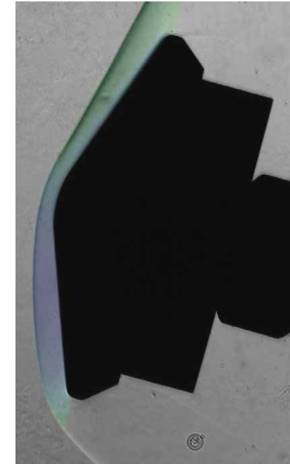
Schlieren image of high-enthalpy CO 2 flow over Mars Science Laboratory geometry.
