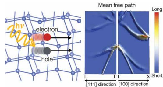
This illustration depicts dynamics of excited electrons during the first picosecond (millionth of a millionth of a second) after sunlight is absorbed in a silicon solar cell. Shown on the right is the average distance excited electrons travel before losing energy to heat. This distance, called mean free path, is calculated for electrons with a range of energies and moving in different crystallographic directions.
