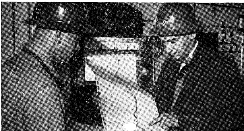
Roger Jones, B.S. in Chem., Haverford College '52 (right), and operator check temperature control in the conversion of furfural to furan.
