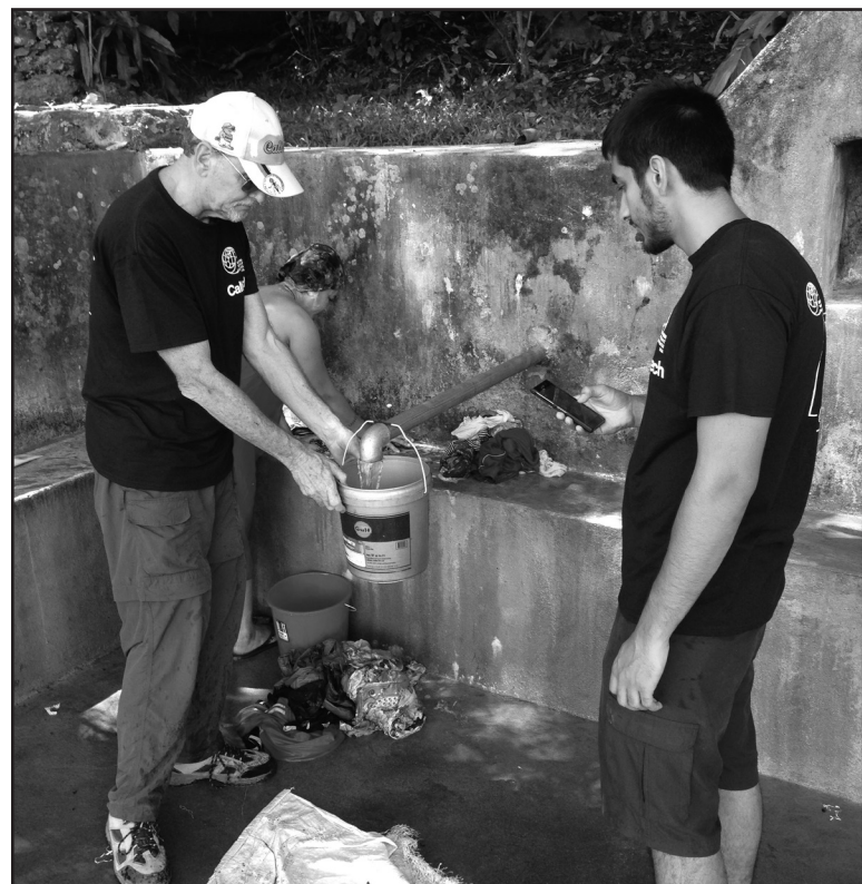
Gordon Treweek and Nauman Javed measure the flow rate of the spring.
