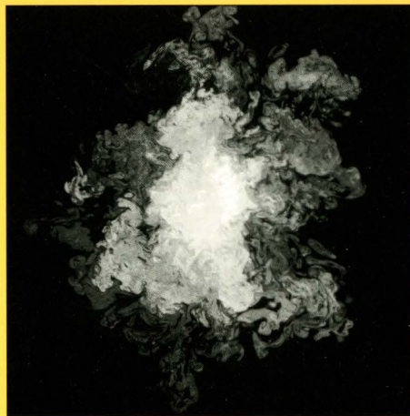
This image, produced with laser-induced fluorescence techniques, shows a jet-fluid concentration 275 jet-nozzle diameters downstream from the discharge nozzle. Black areas denote the fluid into which the jet is discharged. White indicates the region of highest concentration; regions of lesser concentration are gray.
