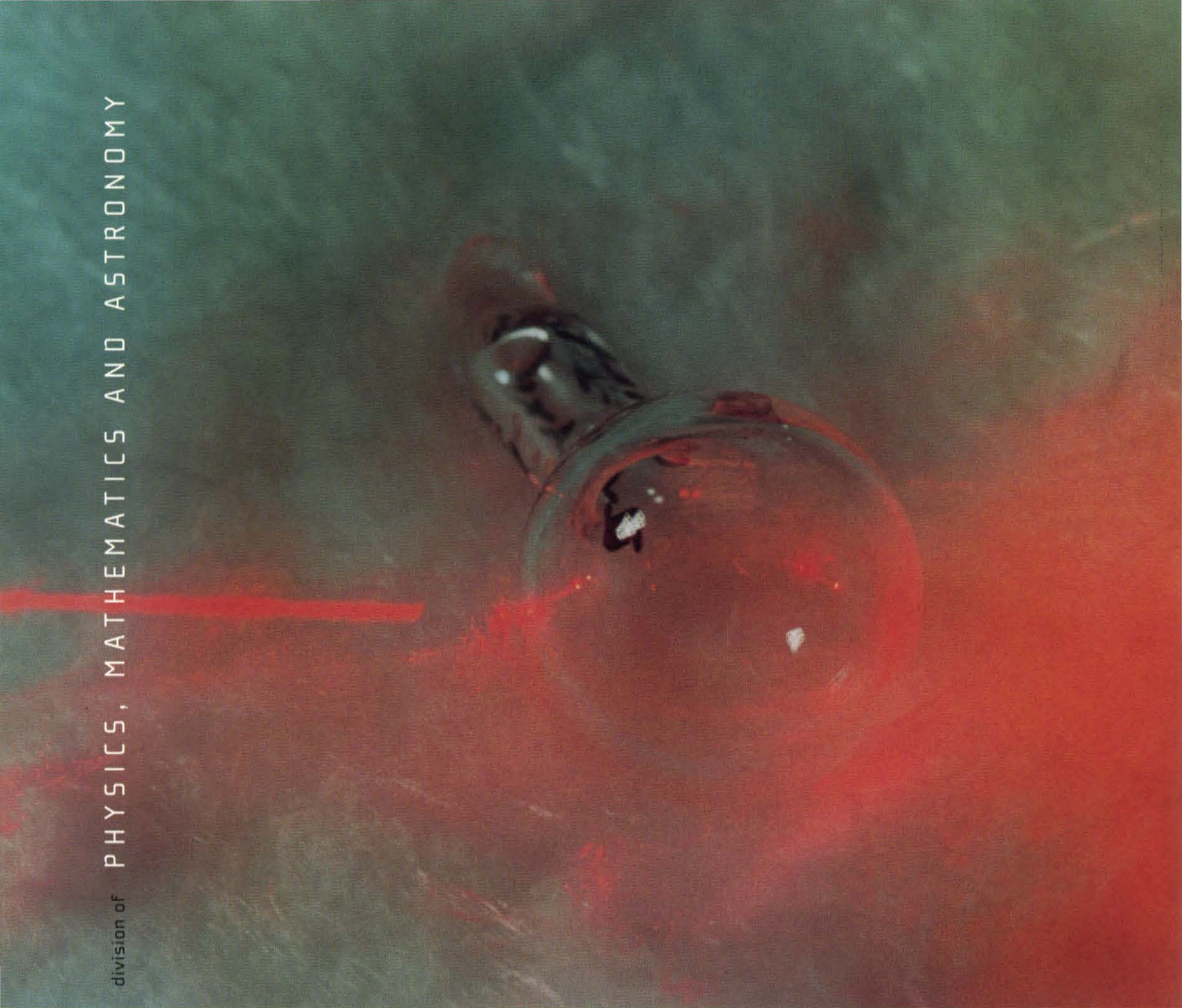
Photographic [above] and MRI [left] images of a glass cell containing low-field polarized noble gas.
