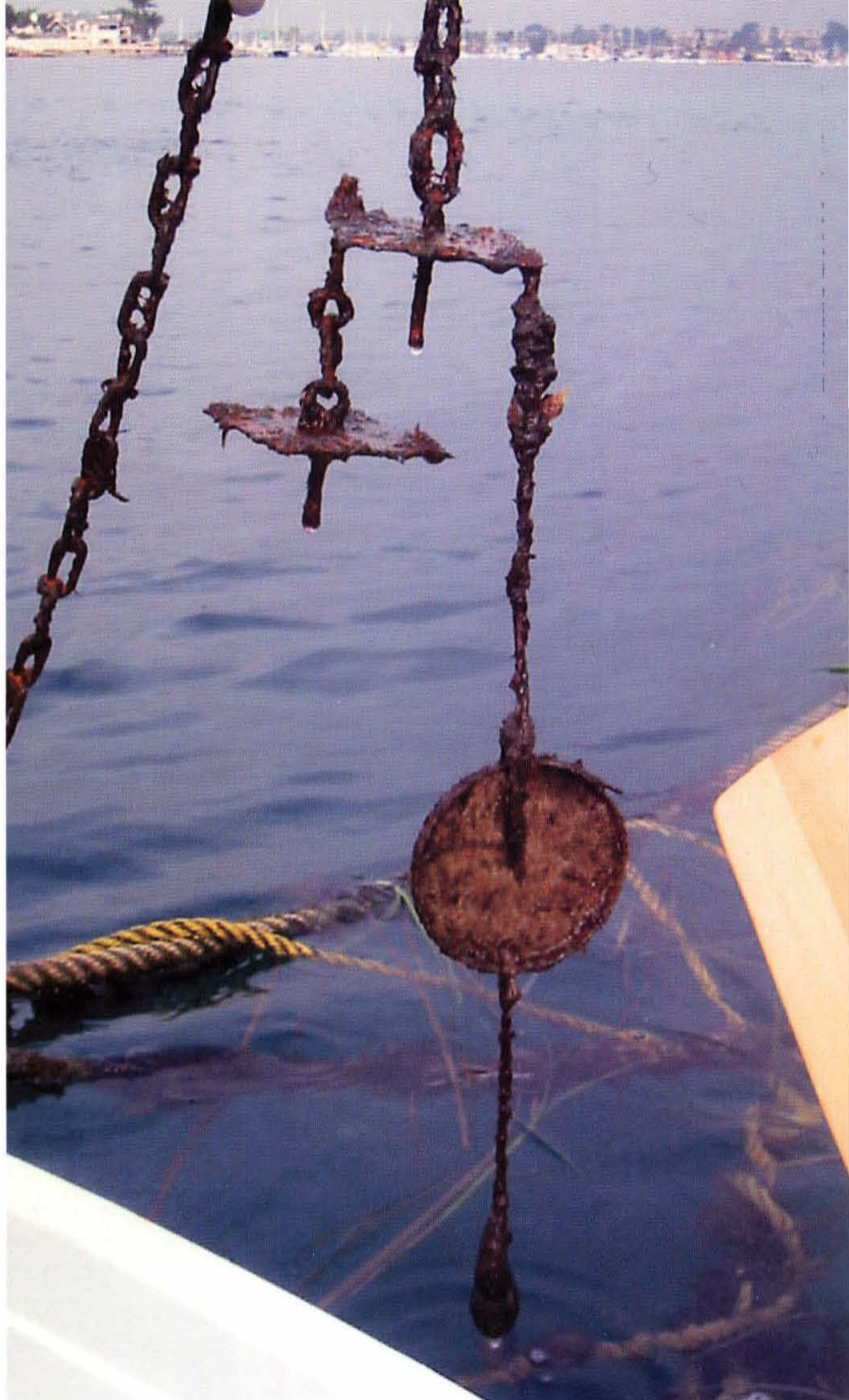
[color images] Biofilms on a recovered piece of carbon steel that was suspended in the waters off Caltech's Kerckhoff Marine Laboratory. [b/w images] Scanning electron micrographs of Shewanella oneidensis strain MR-1 in a biofilm attached to the surface of carbon steel.
