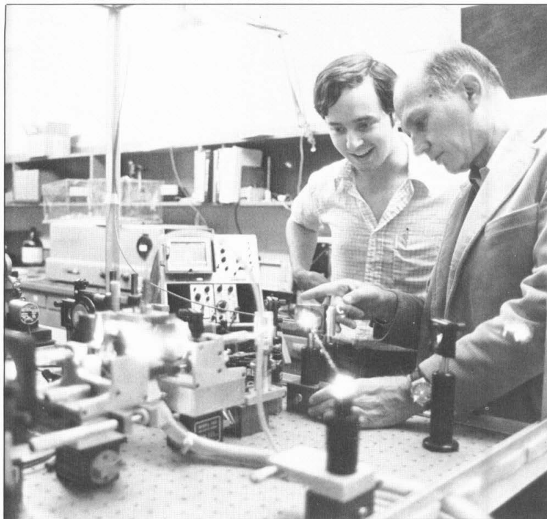
Dr. Amnon Yariv and graduate student Tom Koch make adjustments on a dye laser and amplifier system capable of producing a continuous stream of gigawatt peak power optical pulses with durations of one picosecond ( 10^{-12} s). This system is used to study ultrafast processes and switching phenomena in semiconductors.
