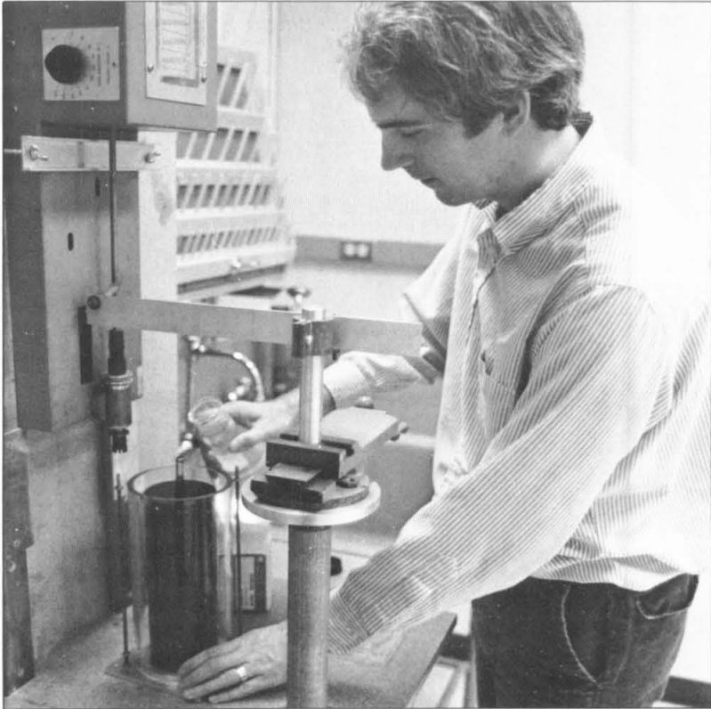
Assistant Professor of Chemical Engineering Eric Herbolzheimer prepares a couette flow device used to measure the sedimentation velocity of particles in sheared suspensions.
