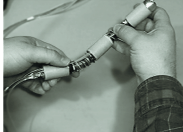
Medical robot prototype. The goal of this device is to access, in a minimally invasive fashion, the portions of the small intestine that cannot be accessed by conventional endoscopes.
