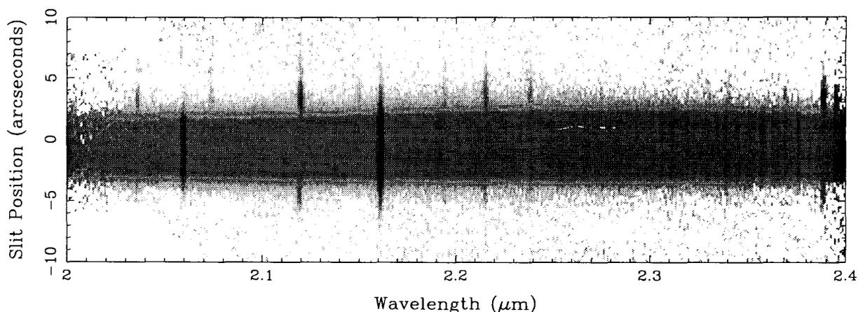
A spectrum of the planetary nebula BD+30 to illustrate the capabilities of the instrument. The spectrum covers the entire K-band atmospheric window with a wavelength range from 2.0 to 2.4 microns. The broad horizontal stripe is thermal radiation from the main shell of material surrounding the remnant of the central star. Thin vertical stripes are individual emission lines due to energy transitions in various atomic and molecular species within the shell and surrounding material.
