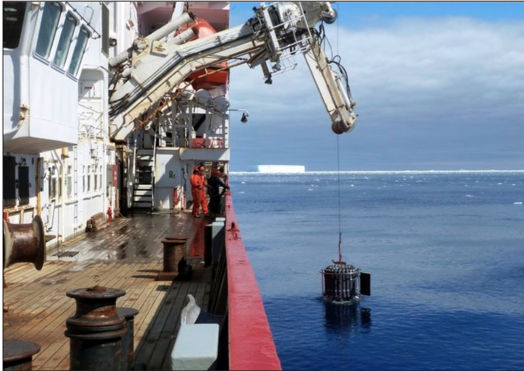
The team lowers machinery for measuring conductivity, temperature, and depth into the ocean.
