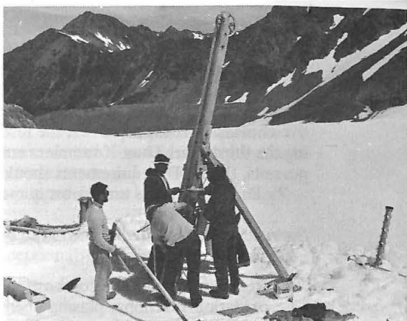
Students and staff prepare drilling equipment for deep coring in ice, Blue Glacier, Washington
