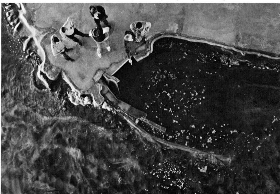
This man-made three dimensional model at Caltech's Azusa laboratory is used in research concerning the behavior of waves in harbors. Like tall buildings in earthquakes, harbors respond to stress from wave action in differing ways. Fredric Raichlen, professor of civil engineering, and Vito A. Vanoni, professor of hydraulics, emeritus, are principal investigators.
