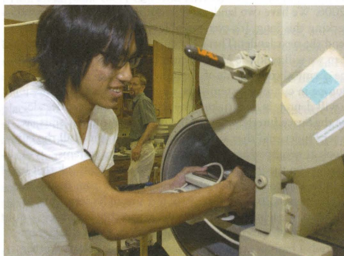
Nathan Chan '08 (the Carolyn Ash SURF Fellow) loads a scale into the airlock of an oxygen-free glovebox in order to weigh chemicals that react quickly with oxygen. In his SURF project, "Oxidation States of Trace Elements and Their Effects on Water Chemistry around Lake Powell," Chan worked with Caltech professor Janet Hering, an aquatic chemist, and graduate student Richard Wildman.
