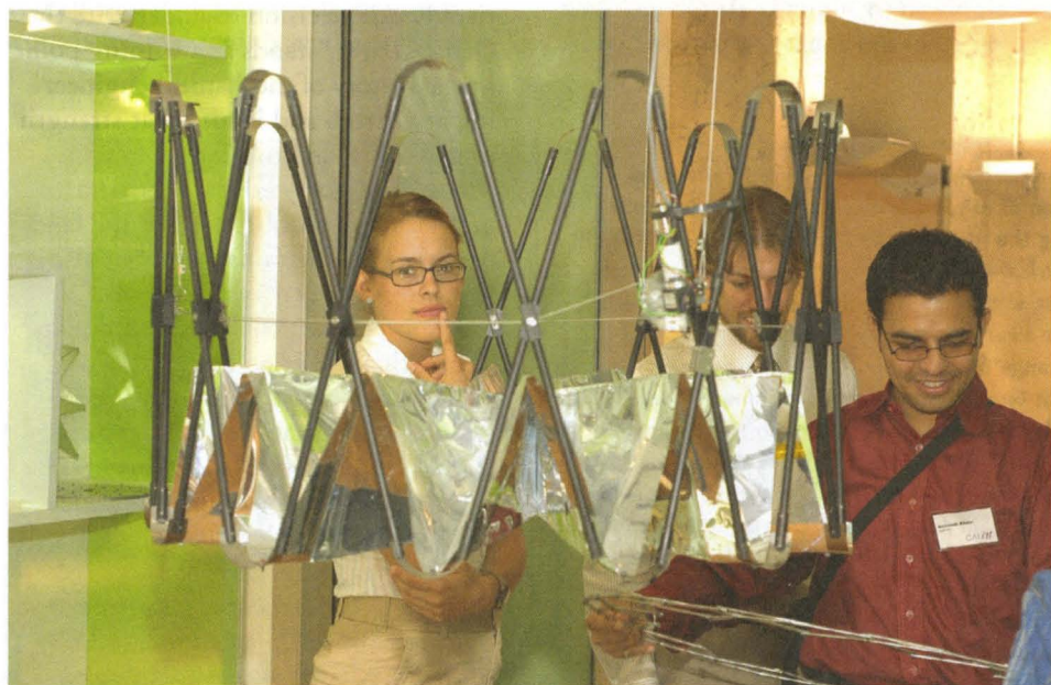
Expandable science: in the new Space Structures Laboratory, graduate students (left to right) Gwendolyn Johnson, Jeff LeHew, and Dev Khatri examine models of structures that can be deployed and collapsed as needed by spacecraft.
