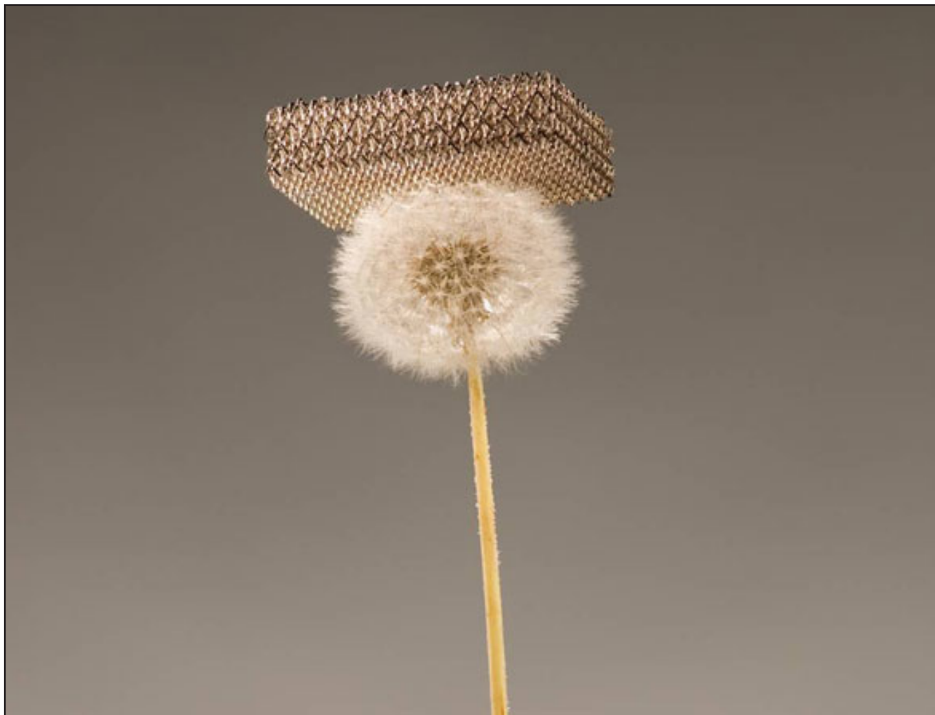
The ultralight metallic lattice displayed above is easily supported by a budding sunflower.
