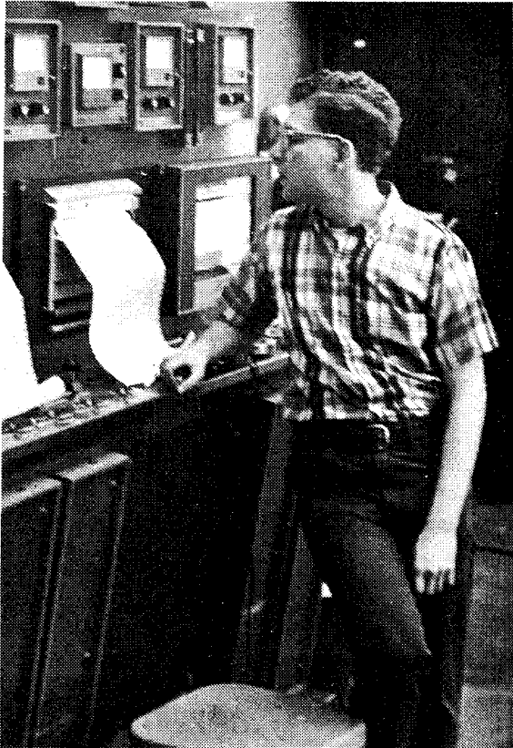
Disconnecting the vacuum spark advance on older model cars has been suggested as a way to reduce their emissions, and hence help control smog. However, GM claims that disconnecting the advance will cause cars to overheat. To test this contention, the Caltech Clean Air Car people have been conducting their own test, using cars volunteered by members of the Caltech community.
